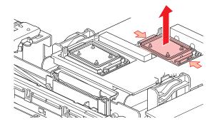
**5** [When using Sb ink and TP ink] Rinse the cap with the mesh side facing downward in a container filled with maintenance liquid. Remove, then wipe clean the resin part thoroughly.
