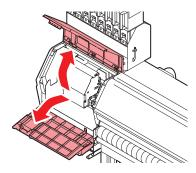
**2** Remove the side screw, and detach the media holder stopper.
