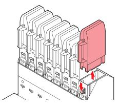
**2** Remove the ink absorber, and replace with a new one.
